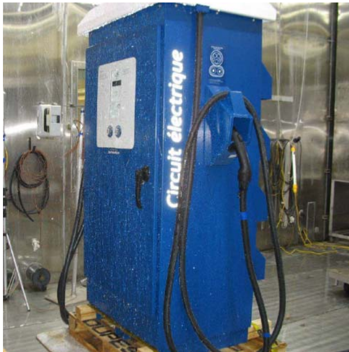
Heavy rain test
